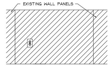
ATTACH PANEL TO THE WALL. PANEL SHOULD CLEAR EXTENSION. SCREW INTO PLACE LARGER OUTLET COVER THAN ORIGINAL AND RESTORE POWER TO THE OUTLET.
