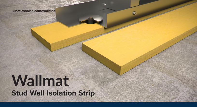
Kinetics Noise Control's Wallmat resilient partition isolation pad is a custom molded fiber glass board which resiliently decouples a sound-rated partition from non-isolated structure. Isolation is maintained with the use of KAI which isolates fasteners. Apply Wallmat continuously along the bottom and top plates of a stud wall wherever acoustical isolation is required to maintain a fully effective sound rated assembly.
