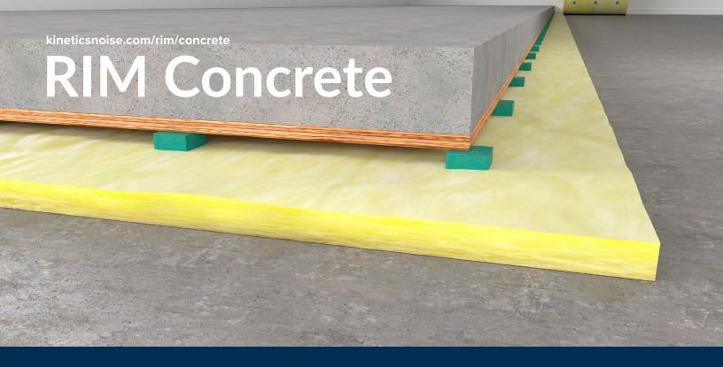
RIM is a high-performance noise control system that is easily installed. The rolls of RIM use acoustic batting to prespace isolation pads. These pads form an airspace—an essential component for noise control.
